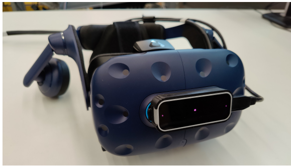
Figure 2: The HTC Vive Pro Eye VR headset used in the study, with the Leap Motion hand tracking sensor mounted on the front. The setup allows for continuous hand tracking as the user operates in the VR space.
