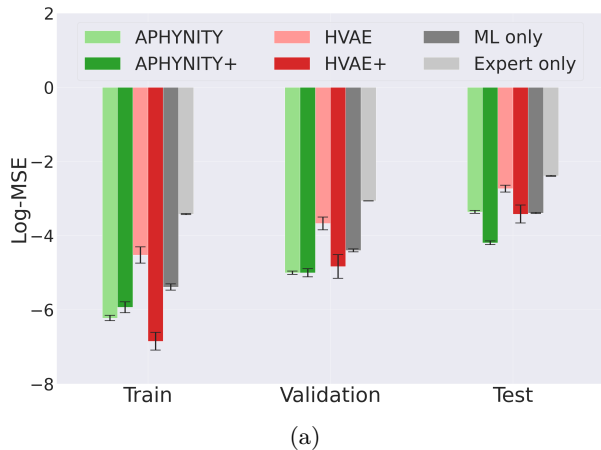
Figure 9: The results of the double pendulum experiment. (a) The average log-MSEs over three experiments. The baselines rely either only on the expert ODE or a neural ODE to predict the pendulum’s state. The proposed expert augmentation slightly reduces the predictive performance on the training set for APHYNITY but increases the generalisation capabilities of both APHYNITY and the HVAE. APHYNITY+ outperforms the baselines on all sets. (b) The average relative errors on the initial angular speeds over three runs. The proposed expert augmentation improves the accuracy of the physical parameters estimation both in the IID and OOD settings for APHYNITY.
