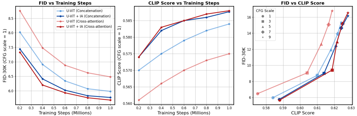
Figure 4: Evaluation during training and FID-30K vs CLIP Score at different CFG scales. settings with IA show improved generation quality and text-image alignment compared to their early fusion counterparts. CLIP Score is measured on 30K pairs using CLIP-ViT-L-14.
