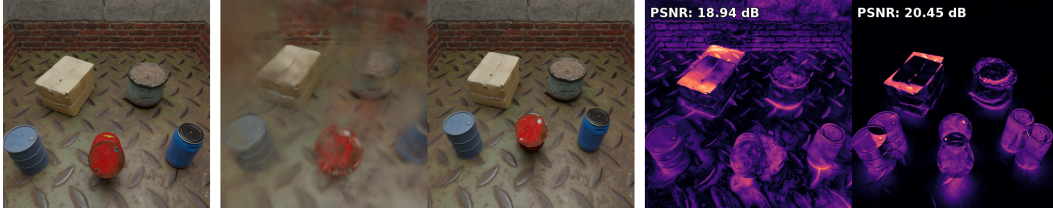
Figure 19: Qualitative comparison of last frame from scene factory of NVFi by only using an autoregressive transformer without the ODE component. From left to right is the GT image, the transformer’s rendered image, the baseline (Yang et al., 2024)’s result, the difference between the GT and transformer’s rendered image, and finally the difference between the GT and the baseline’s rendered image.
