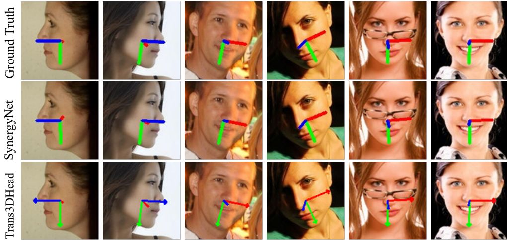
Figure 11: Examples of head pose estimation predicted by the SynergyNet and the proposed Trans3DHead on the AFLW2000-3D dataset.
