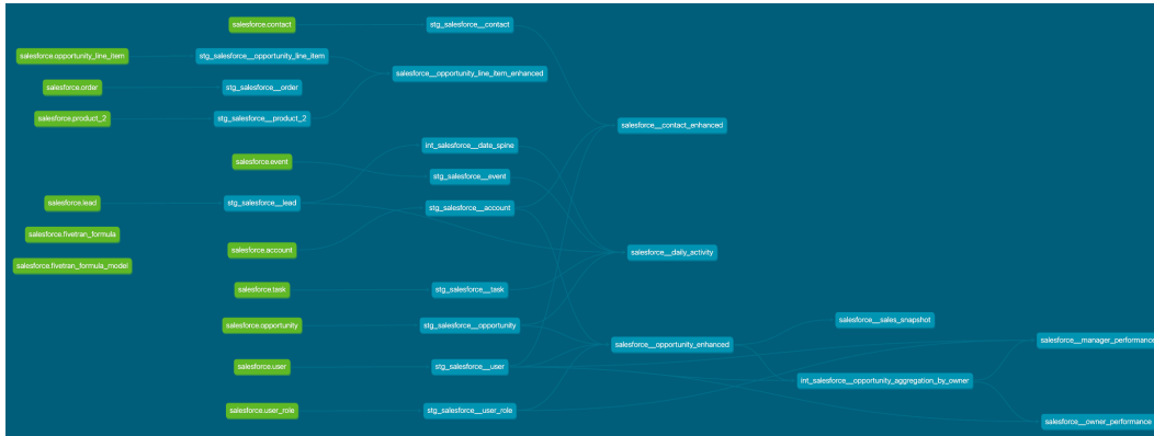
Figure 11: A DAG (Directed Acyclic Graph) illustrating the data flow and dependencies between various Salesforce tables and models in a dbt (data build tool) project. The graph shows stages of transformation, from raw Salesforce data (green nodes) to enhanced and aggregated models (blue nodes), representing different entities such as opportunities, contacts, accounts, and events.
