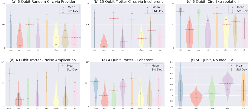
Figure 4: Performance of mitigation methods across various circuit configurations and noise settings. The x-axis displays different QEM methods, while the y-axis represents the absolute error distribution. Panels (a)–(e) use a symlog scale for clearer visualization, as error rates are low after mitigation. Each panel title indicates the specific setting. The width of each violin plot reflects data density at each value, with a broader shape near zero indicating better performance. Our method is shown in red, and raw noisy data is in blue.
