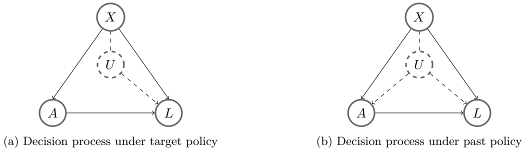
Figure 2: Directed acyclic diagrams representing the causal structure of the decision process under (a) target policy, which yields (3), and (b) past policy, which yields (4). In (b), both contextual covariates (X, U) may joint affect actions A and outcome loss L . Thus U gives rise to unmeasured confounding.
