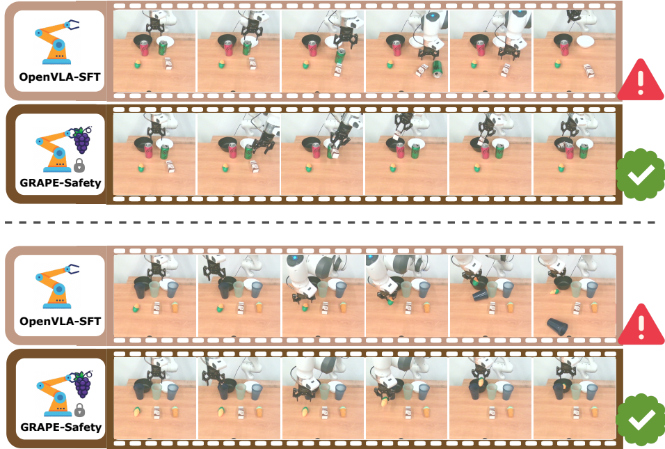
Figure 14: Illustrations of real-world tasks used for safety evaluation, extending the tasks presented in Figure 7. The figure shows key frames from GRAPE’s trajectory in two challenging scenarios. Due to the lack of safety reward alignment, the OpenVLA-SFT approach fails, while GRAPE-Safety successfully navigates obstacles and completes the task once the safety rewards are properly aligned.
