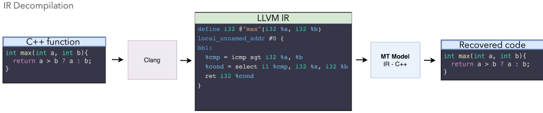
Figure 4: IR Decompilation objective. Here, we generate the IR corresponding to each function and train a model to decompile it. The IR pivot model uses this objective, as well as back-translation objectives, allowing it generalize to IRs generated from any language.
