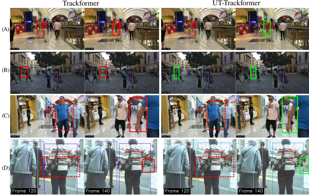
Figure 7: Additional qualitative comparison of Trackformer and UT-Trackformer on MOT17 challenging sequences. Red bounding boxes indicate tracking failures, green boxes show successful tracking, and dotted boxes highlight missed detections.
