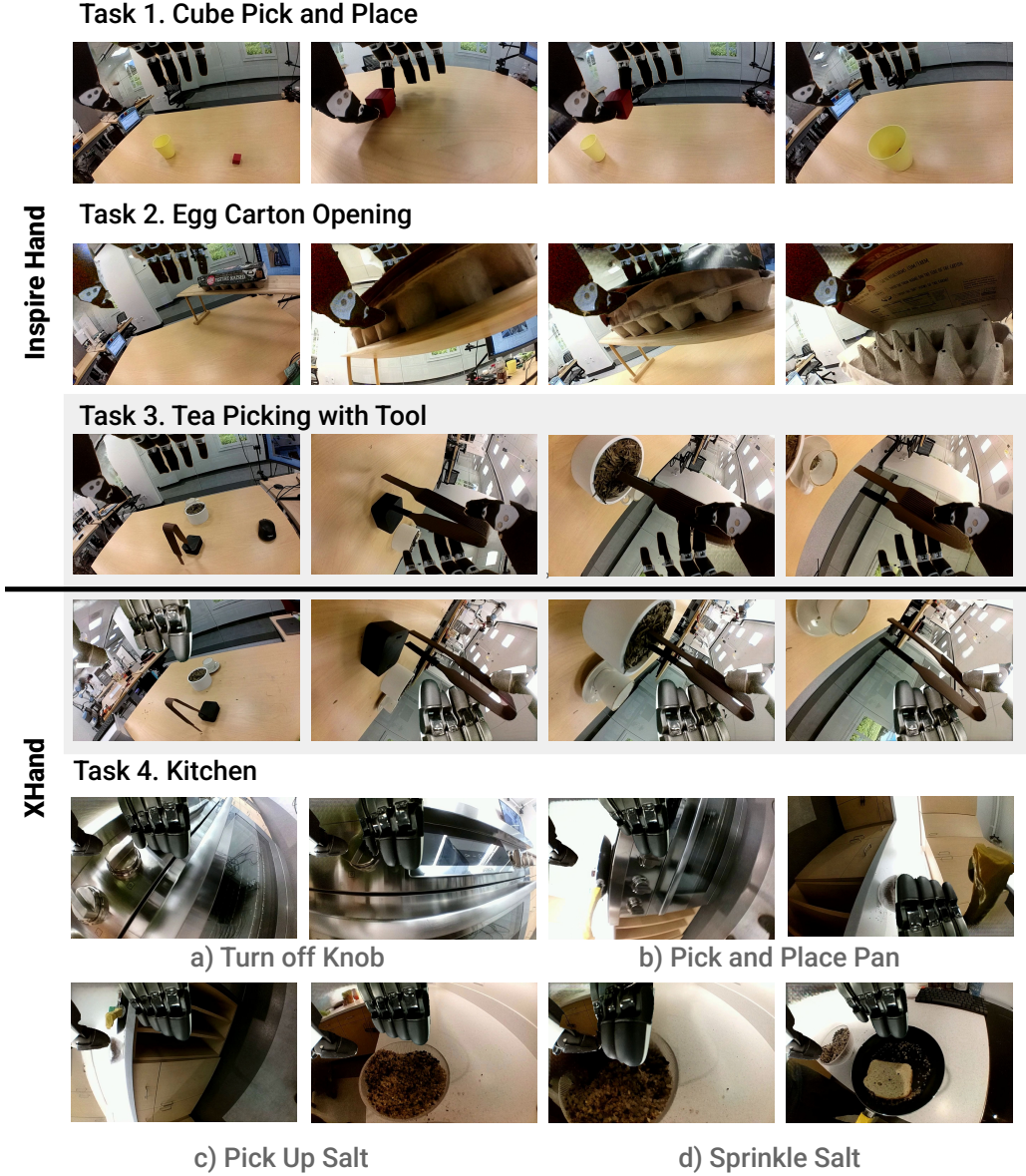
Figure 8: Inpainting Results. The visual observations in the original collected dataset contain exoskeletons and human hands. The software adaptation layer replaces these pixels with corresponding robot hand images while preserving the natural occlusion relationships during hand-object interactions. Please see project website https://dex-umi.github.io for details.
