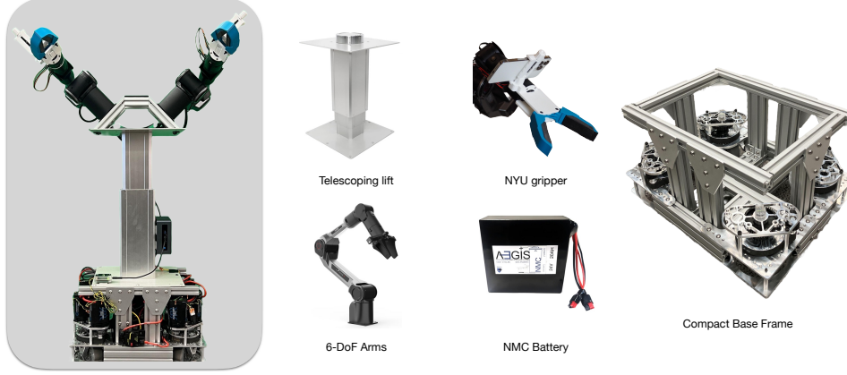
Figure 2: Cone-E is modular and easily customizable with different arms, end-effectors and sensors.
