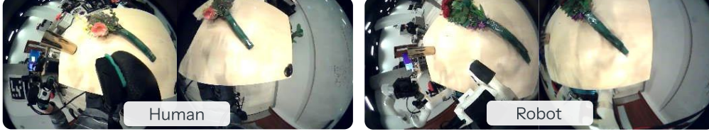
Figure 3: DexWild aligns the visual observations between humans and robots to bridge the embodiment gap. This incentivizes the model to learn a task-centric rather than embodiment-centric representation.
