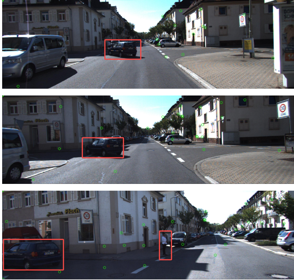
Figure 13: Visualization of the Keypoints-Aware Auxiliary Loss (2). Green points indicate the top-k queries with minimal error relative to the ground truth pose, showing that they are primarily located in regions associated with static objects, while less focus on dynamic objects (red boxes).
