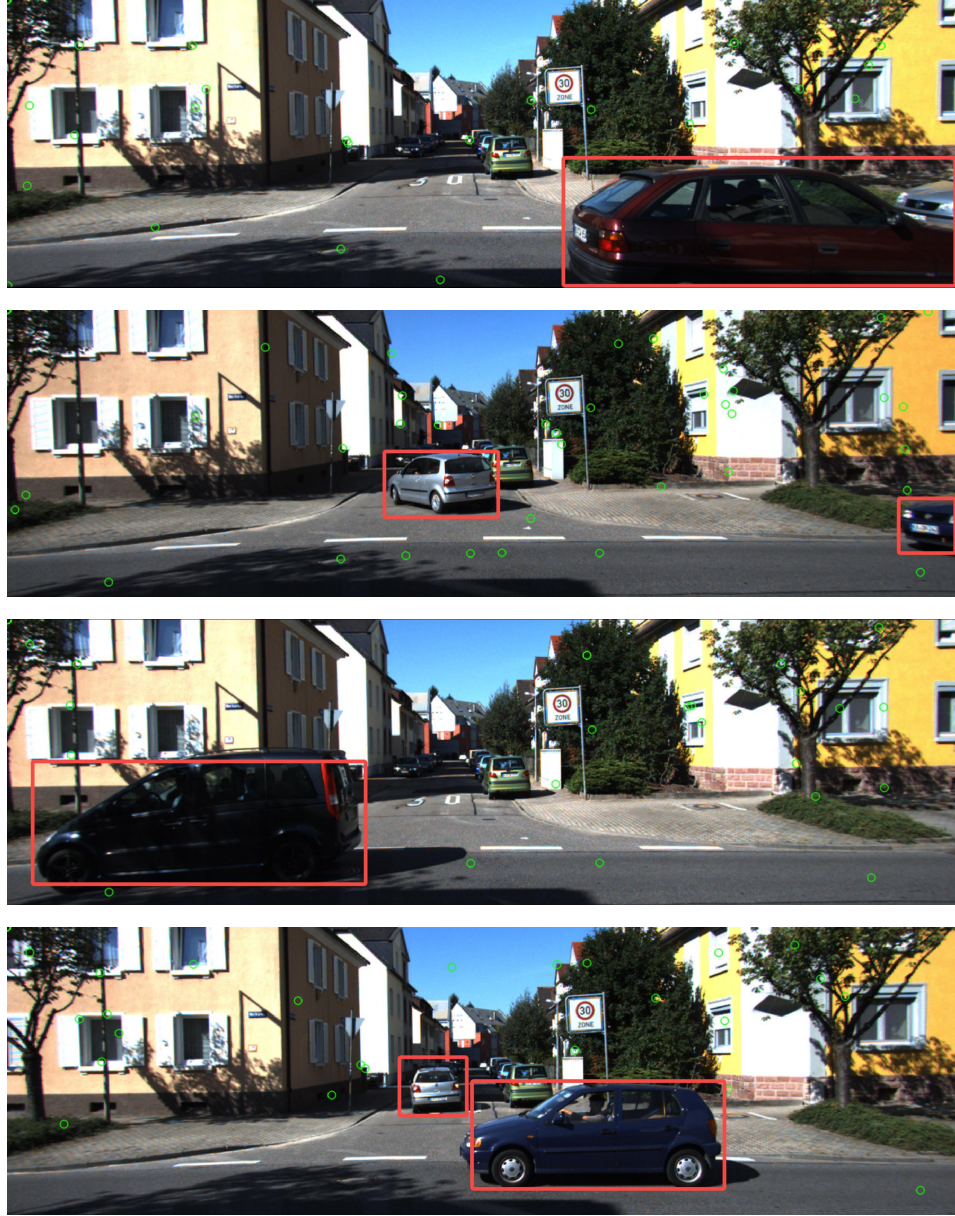
Figure 12: Visualization of the Keypoints-Aware Auxiliary Loss (1). Green points indicate the top-k queries with minimal error relative to the ground truth pose, showing that they are primarily located in regions associated with static objects, while less focus on dynamic objects (red boxes).
