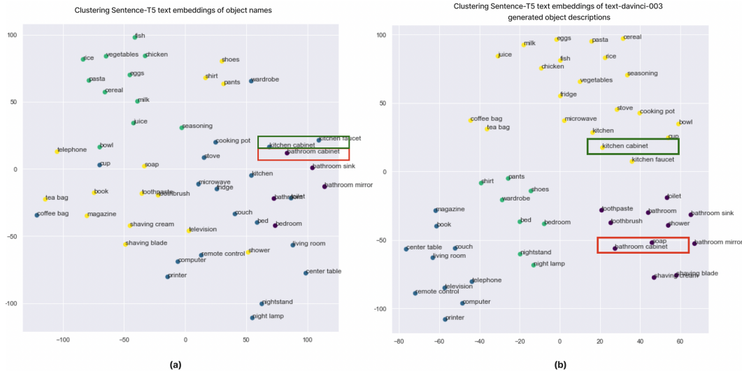
Figure 4: This figure depicts the results of performing k-means clustering on 768-dimensional embedding vectors for each environment object, results are visualized in a 2D latent space. Embeddings for each object in Figure (a) are generated by encoding the shown object name using the Sentence-T5 model. Conversely, embeddings in Figure (b) are generated by Sentence-T5 encoding text descriptions of each object generated by text-davinci-003. The number of clusters used in the k-means algorithm was four(4) based on the number distinct exploration zones in HomeGrid. Note that embeddings generated from LLM object descriptions improved the separation of emergent cluster boundaries, and desirably increased the distance in latent space between similar yet contextually different objects such as Kitchen Cabinet and Bathroom Cabinet.
