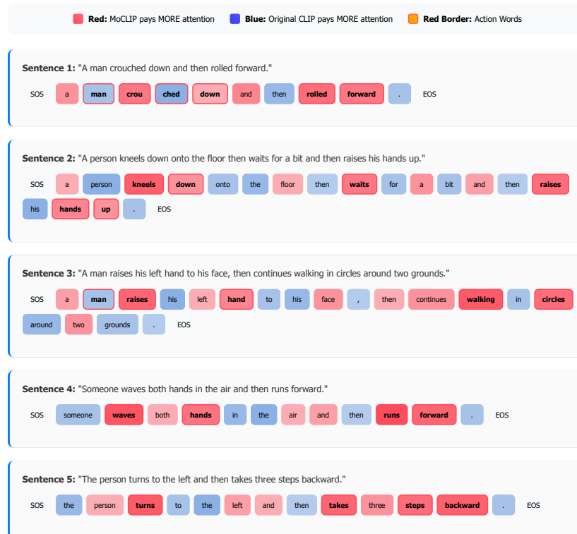
Figure 11: Comparison of final-layer attention between MoCLIP and original CLIP on motion descriptions. Red tokens receive more attention in MoCLIP, blue in original CLIP; red borders denote action words. MoCLIP consistently reallocates attention toward verbs and motion-centric tokens, highlighting its improved focus on the semantic core of actions.
