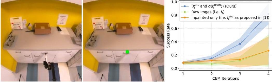
**Figure 5: Real-world experiment setup and results.** (left) Raw views from camera, (center) Inpainted image with agent-agnostic representation (green dot at top-pixel of end-effector). (right) Success rate as a function of CEM iterations.
