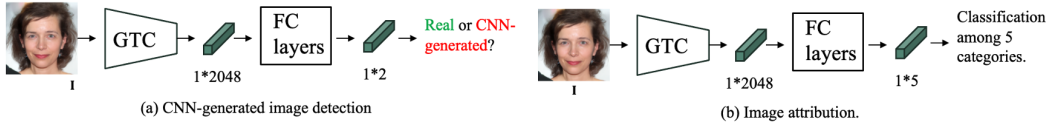
Figure 8: We construct simple classifiers based on GTC. Then, we train these two classifiers for CNN-generated image detection and image attribution, respectively. Please note that GTC only leverages ImageNet pre-trained weights as the initialization, same as the previous method [62]. For a fair comparison, no model parsing datasets such as RED116 and RED140 are used for pre-training.
