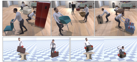
Figure 9. (Top) FORCE generalizes to unseen shapes, demonstrated via pushing, carrying, and pulling. (Bottom) FORCE generalizes to different locations, performing one-handed and two-handed carry from the table and from the floor.
