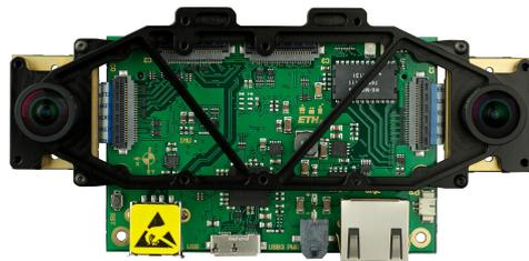
Fig. 1. The sensor hardware used in the experiments: Synchronized data from the global shutter camera and the IMU is streamed to the onboard Intel Atom as well as to external devices via GigE/USB3. The presented experiments used only the data from one camera only.
