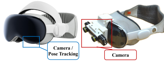
Figure 2: Consumer-grade Devices for Data Collection. To avoid relying on specialized hardware for data collection to make our method scalable, we design our data collection process using consumer-grade VR devices.
