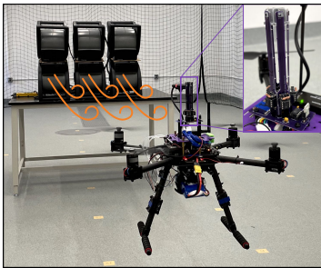
Figure 1: FlowDrone calculates fast and accurate wind estimates with the MAST (inset) to achieve superior flight performance in gusty conditions.
