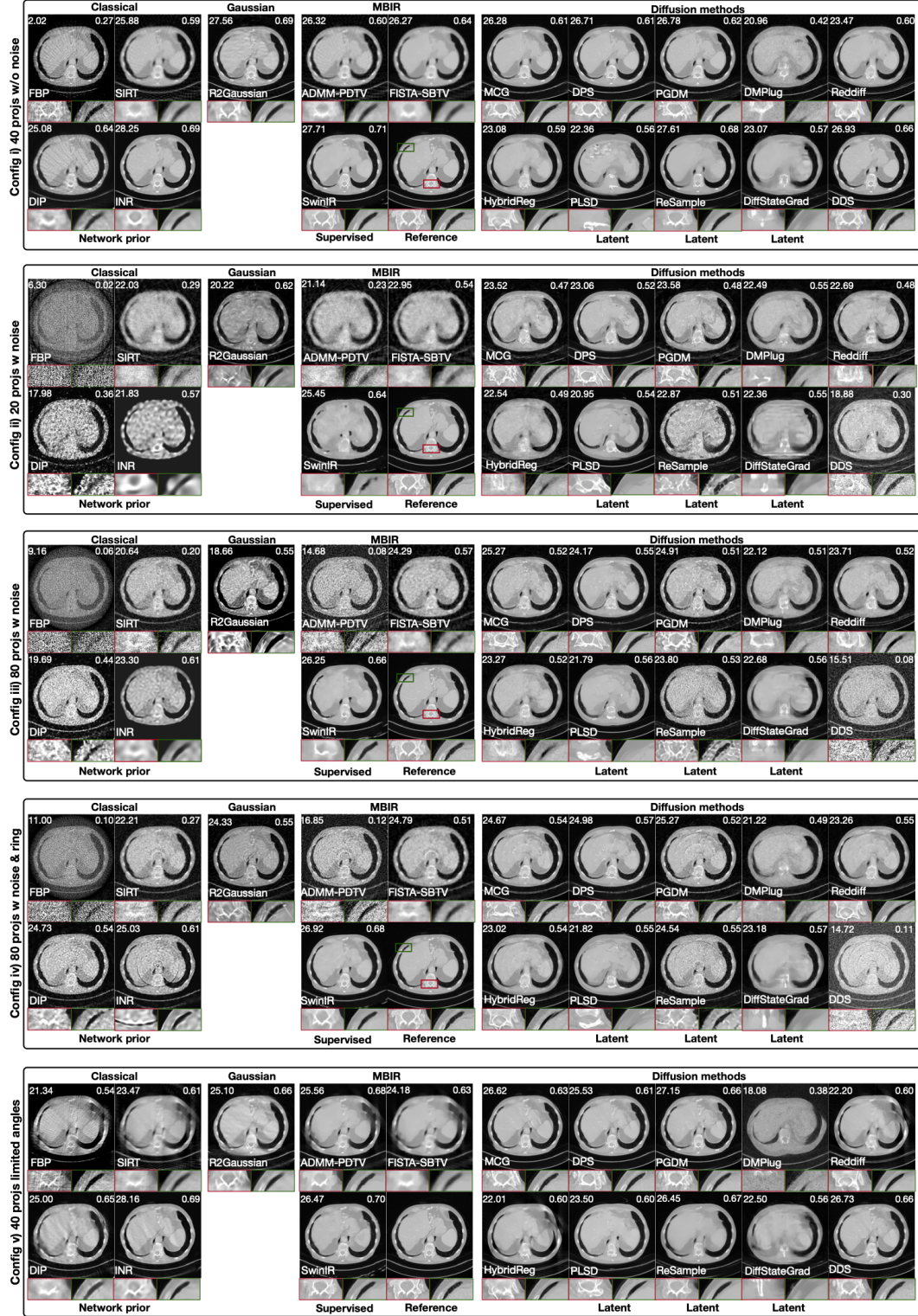
Figure 19: Visual comparison of all benchmarked methods on the simulated medical CT dataset under four different configurations: (i) 40 projections without noise, (ii) 20 projections with mild noise, (iii) 80 projections with stronger noise, and (iv) 80 projections with noise and ring artifacts. PSNR and SSIM are shown in the top-left and top-right corners. Red and green insets highlight zoomed-in regions.
