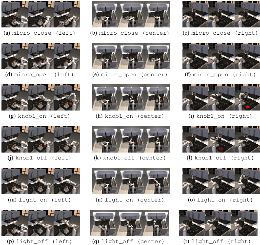
Figure 9: Initial frame (Easy), initial frame (Hard), and goal frame for all 12 tasks and 3 camera views in our FrankaKitchen suite.
