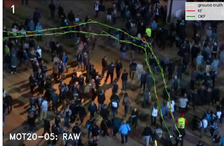
Figure 5: A sample of 2 trajectories in the first frame of MOT20 test video, along with the predictions of KF and OKF.
