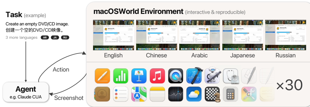
Figure 1: macOSWorld is an interactive computer-use benchmark, allowing GUI agents to operate in a real macOS environment and complete a series of tasks. To facilitate multilingual benchmarking, both the tasks and the environments are provided in 5 languages.
