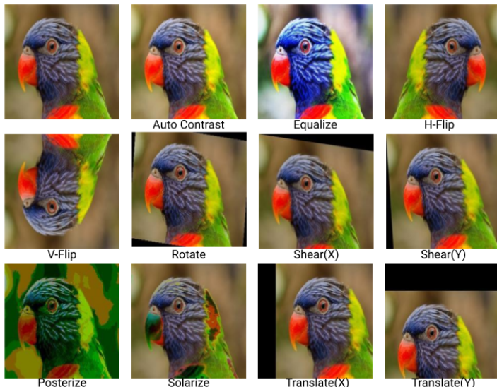
Figure 5: Augmentations used for Dynamic Mixup with 11 operations. We increased some operation intensities for illustration purposes.
