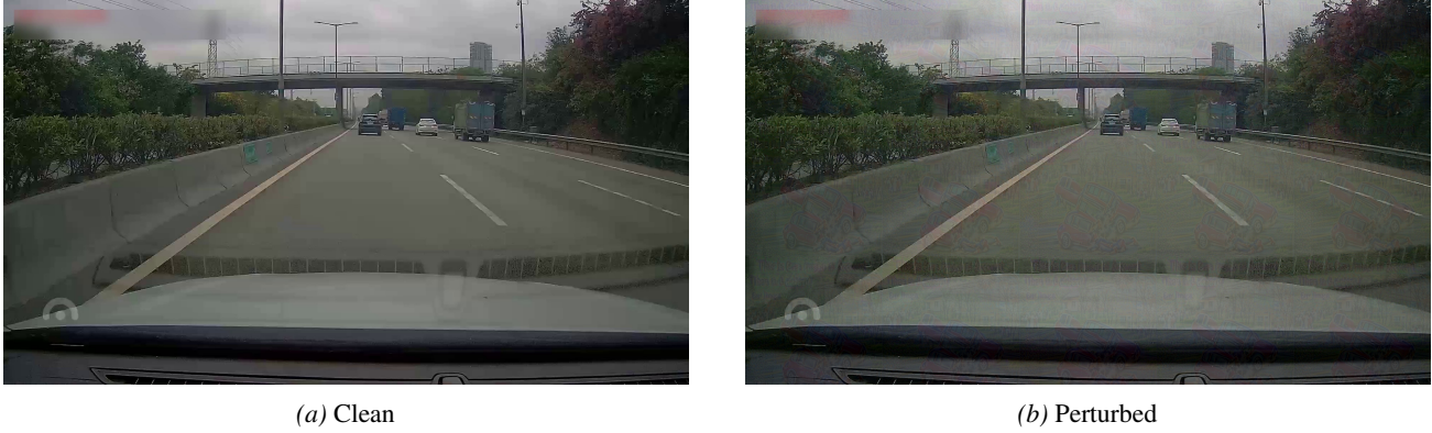
Figure 8. Example D 2 -City frame before and after applying the XTransfer UAP ( \epsilon = 12/255 ). The tiled structure arises from spatially repeating the 384 \times 384 UAP to match the input resolution. The perturbation is largely imperceptible at the applied \epsilon .
