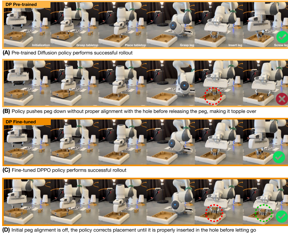
Figure 6: Qualitative comparison of pre-trained vs. fine-tuned DPPO policies in real evaluation. (A) Successful rollout with the pre-trained policy. (B) Failed rollout with the pre-trained policy due to imprecise insertion. (C) Successful rollout with the fine-tuned policy. (D) Successful rollout with the fine-tuned policy that requires corrective behavior.
