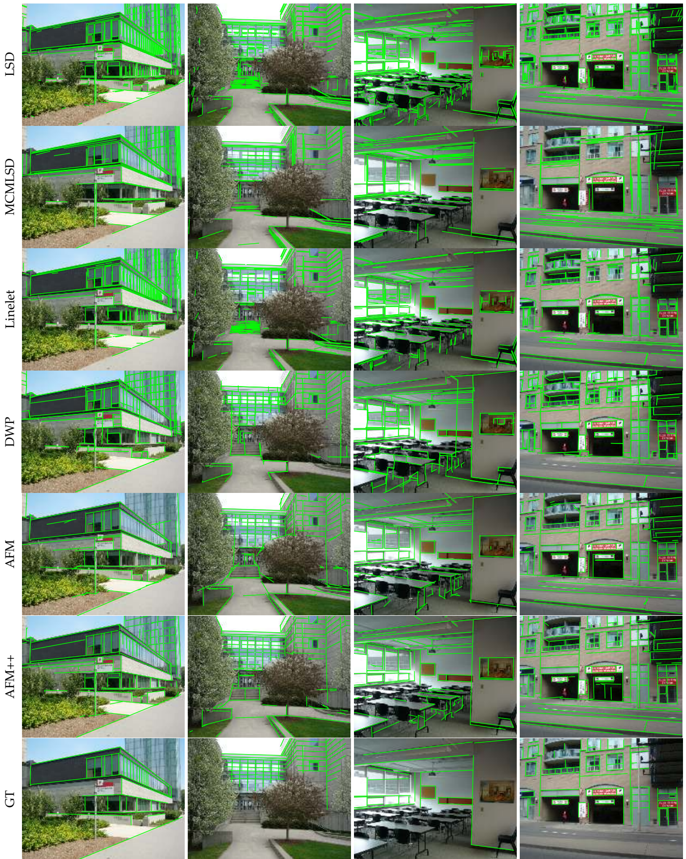
Fig. 8. Some results of line segment detection of different approaches on the YorkUrban [4] datasets. From top to bottom: LSD [2], MCMLSD [3], Linelet [18], DWP [12], AFM [33] with the a-trous Residual U-Net and AFM++ proposed in this paper.
