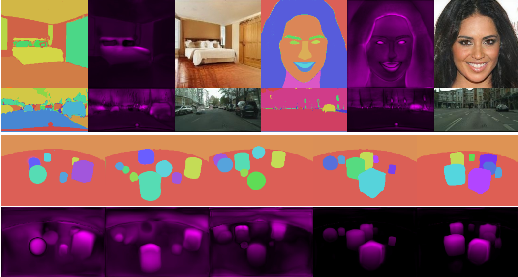
Figure 2: Layout and image generation. The GANformer2 model generates each image by first creating a layout that specifies its outline and object composition, which is then translated into the final image. While doing so, the model produces depth maps of the object segments which are used to determine their relative ordering, and notably are implicitly derived by the model from the layouts in a fully unsupervised manner.
