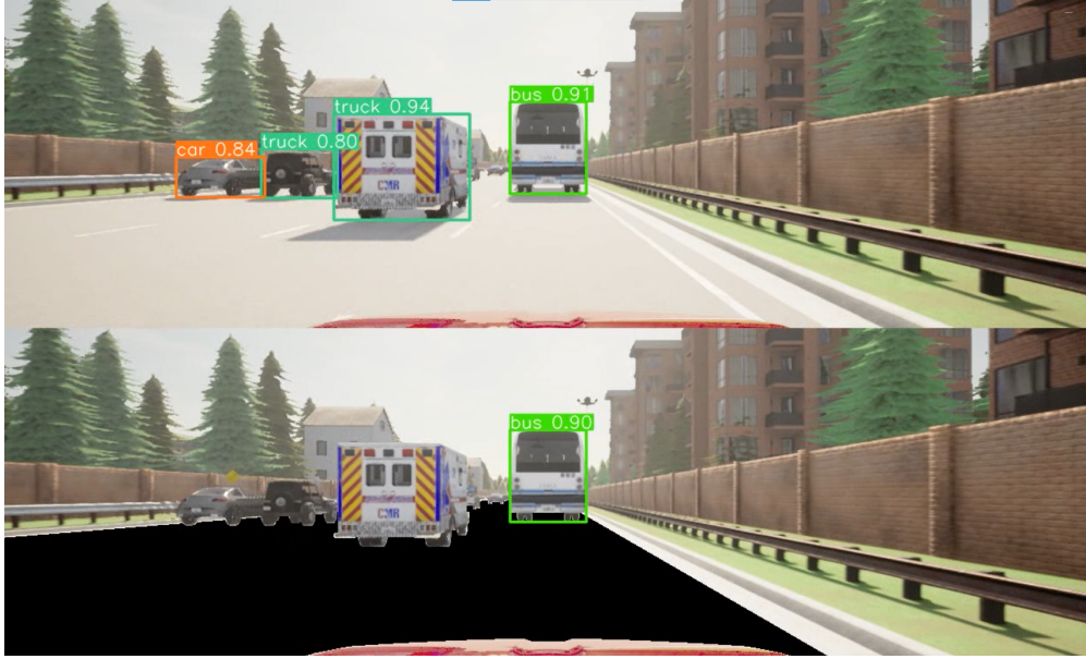
Figure 4: Masking the road on CARLA image and generating inference using YOLOv8 model. Top: 3 out of 4 vehicles are correctly detected. Bottom: road-masked image, where only one vehicle is detected.
