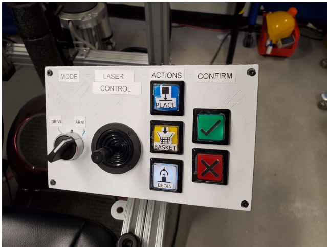
Figure 3: The control panel for the SAR UI. The cursor is controlled by a joystick, and the buttons can light up to indicate what actions can be taken from a given state. Audio prompts are played through speakers that guide the user through using the interface.
