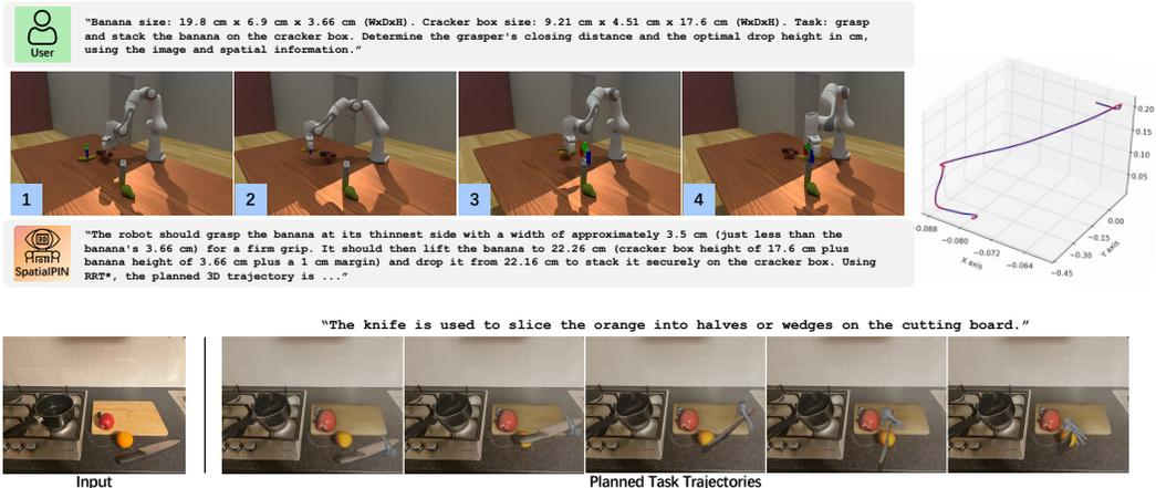
Figure 5: **Qualitative examples of pick and stack (top) and task trajectory planning (bottom).** SpatialPIN successfully outputs picking and stacking policies using spatial reasoning and plans 3D trajectories with geometric awareness to align with task descriptions.
