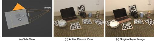
Figure 3: Our method of **partial 3D scene reconstruction** (a). The reconstructed scene (b) and the input image (c) show high alignment.
