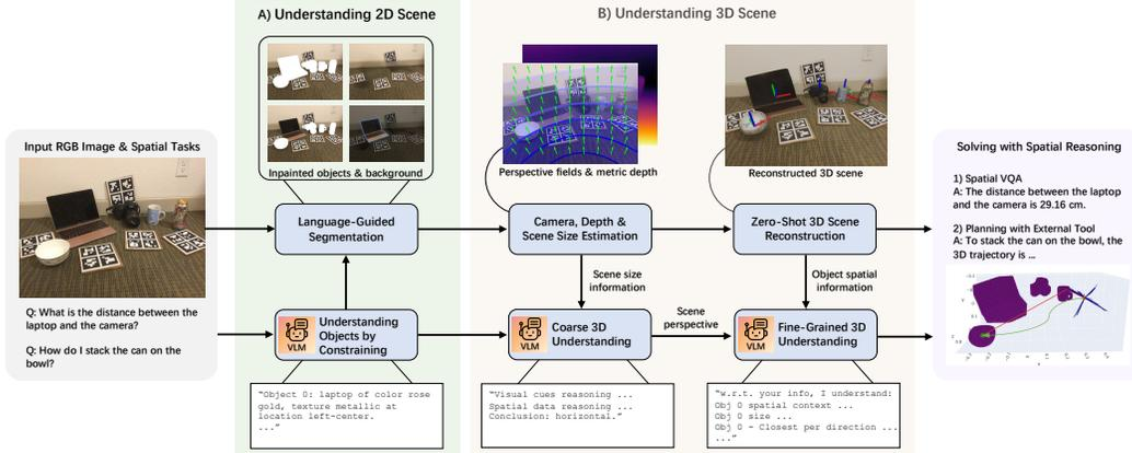
Figure 2: **SpatialPIN**. Our plug-and-play framework is fully modularized and designed for zero-shot deployment. Each module can be easily replaced with the latest updates. Exact prompts for VLMs are in [Appendix](#).
