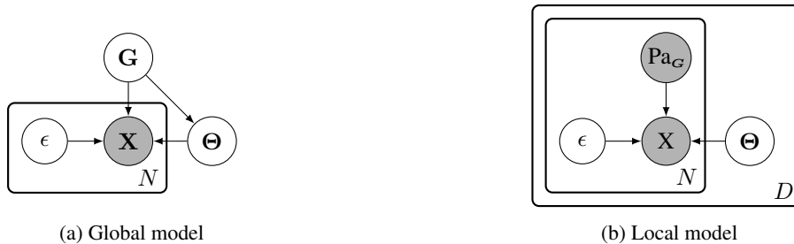
Figure 1: Graphical models for Bayesian CSL. The unobserved exogenous noise \epsilon is included for clarity, but typically modeled by the observational distribution in Equation 12. (a) At a global scale the influence of the causal graph G on parameters \Theta and observed random variables X is emphasized. (b) At a local scale the modularity of the FCM becomes evident. Here, Pa_G denotes the parents of an observed random variable X_d according to some fixed causal graph G .
