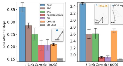
Figure 2: Left: results for *1-Link Cartpole*. Right: results for *3-Link Cartpole*. For all bar charts in this paper (unless otherwise stated): the vertical axis denotes the best loss value after 1,000 optimization steps; the bars show means over 10 runs (for each method), with 90% confidence intervals. Each optimization step runs one simulation episode, computes the loss, and propagates the gradient w.r.t. optimization parameters for algorithms that use gradients.
