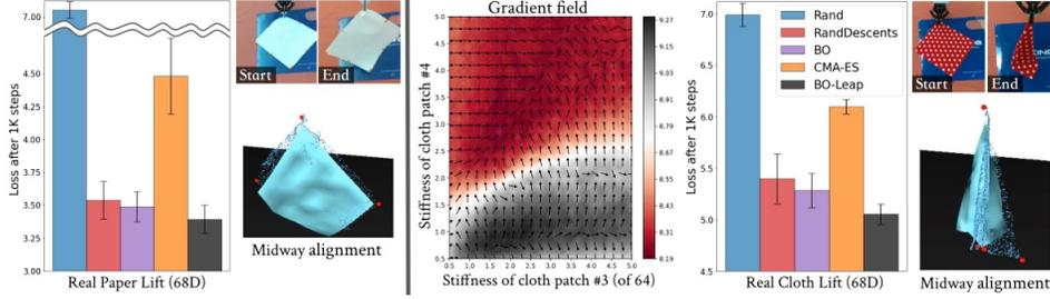
Figure 7: Results for optimizing a simulated object to match the motion of a real paper (left) and cloth (right), which are lifted by a real robot. We visualize the midway alignment showing that our method finds the size, mass, friction and stiffness (for each of the 64 patches) to bring simulated object behavior close to the real one.
