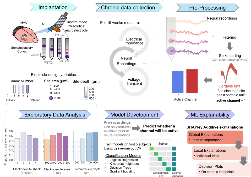
Figure 1: Data collection and Explainable Machine Learning Pipeline. Implantation: A silicon microelectrode with a custom design was implanted in the S1 of rats. The electrode-sites of this device are combination of are shank, area, and depth. Chronic data collection: electrochemical features and neural recordings were obtained for up to 15 weeks post-implantation. Pre-processing: following offline sorting, channels that had sortable units were deemed active. EDA: Percentage of active sites across electrode design variables. Model development: in order to predict whether a channel will be active prior to the recording session, only features available prior to the collection of neural recordings were selected, such as the channel’s previous sortable unit metrics. The development set used to train each classifier was done using leave-one out cross-validation and performance was evaluated on an external validation subject. ML Explainability: SHAP values were computed to determine the most important predictors for the model, on chronic timepoints, and for individual trials.
