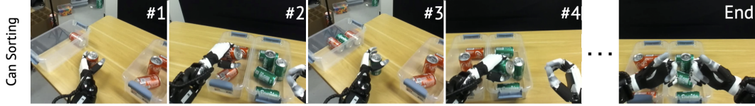
(a) The robot picks up a randomly placed can (#1), places the red can in the left case (#2), picks up the next can (#3), places the green can in the right case (#4). When the sorting box at the edge of the table is empty (as shown in #1, #3) and there is no more can on the table, the robot poses the ending gesture ( End ).
