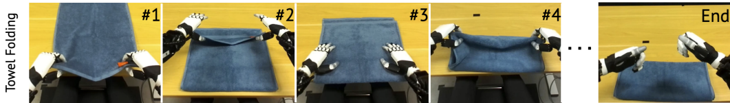
(d) The robot picks up the two corners of the towel (#1), folds the towel (#2), gently moves the towel to the edge of the table (#3), folds the towel twice (#4). When the towel has been folded into a satisfactory configuration, the robot poses the ending gesture ( End ).
