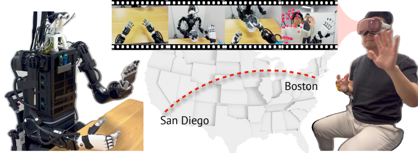
Figure 11: Our system enables cross-country teleoperation over the internet. The operator at Boston, USA can operate a robot at San Diego, USA (approximately 3000 miles away). The robot and operator pictures are flipped left to right for better illustration.
