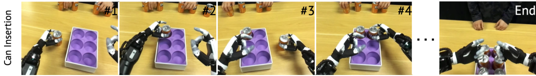
(c) The robot picks up the can (#1), inserts the can into the slot (#2), uses the other hand to repeat picking and inserting(#3, #4). When all six slots have been filled, the robot poses the ending gesture ( End ).
