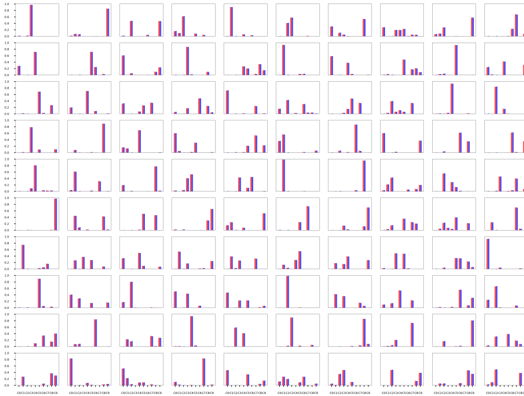
Figure 9: Histogram representation of p(y|s) as well as its server-side reconstruction for every client s for the Cifar10 setup described in Appendix A. The x-axis per sub-plot enumerates the 10 classes. For every class c , the left bar in red represents p(y = c|s) and the right bar in blue represents its reconstruction. Each client performed a single full data-set update step.
