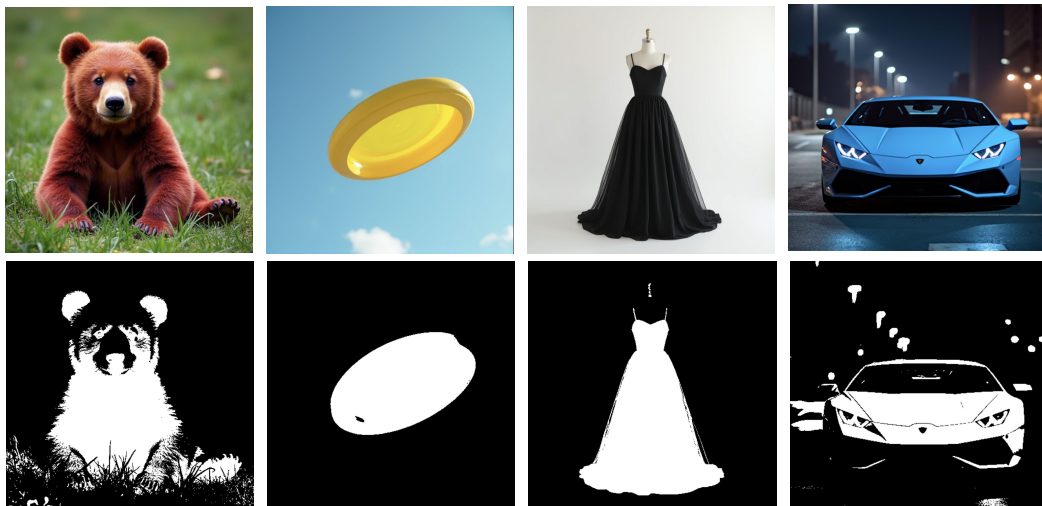
Figure 20: Masks generated by classifying each pixel based on whether its color is closer to that of the central pixel or to the average color of pixels along the side edges. With enough prompts featuring objects in diverse and clearly distinct colors, this method could serve as an alternative to SAM for finding ground truth to select the appropriate cutout head.
