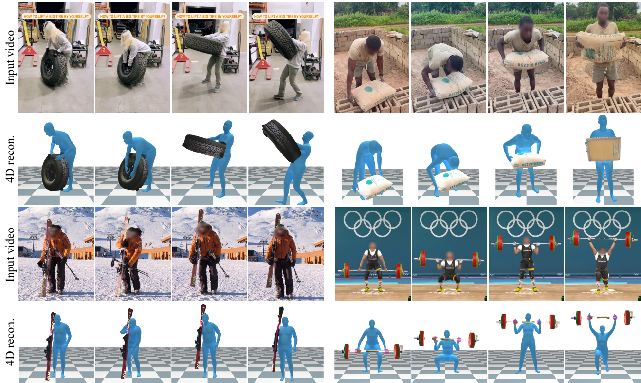
Figure 1. Category-agnostic 4D interaction reconstruction. From a monocular RGB video, CARI4D reconstructs a metric-scale object mesh, tracks human and object motion over time, and predicts coherent hand-object contacts for categories unseen during training.
