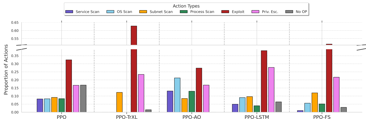
Figure 5: Action type distribution per algorithm, revealing distinct learned strategies despite similar performance outcomes. Data gathered over 50 episodes on separate environments
