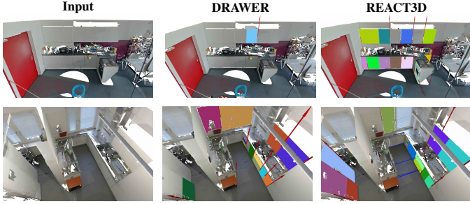
Fig. 3. Qualitative comparison. Red and blue arrows denote revolute and prismatic joints. Our method outperforms DRAWER on handle-less objects (top) and correctly classifies prismatic drawers that DRAWER mistakes for revolute joints (bottom).
