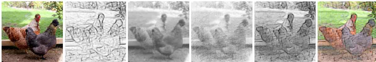
Figure 4: Visualization of the conversion of a real image to a colored pencil drawing. We display, in the following order, the original image, its pencil stroke representation s , the tone map j , the tonal texture t , the grayscale pencil sketch r and the final image.
