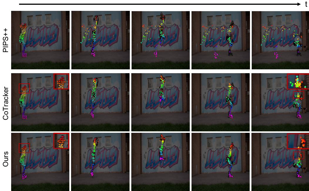
Figure 6: Motion Comparisons. The 2D projected motion of Gaussians accurately aligns with dynamic human motion trajectory in the video, where the point trajectories estimated by PIPS++ [65] tend to get “stuck” in the background wall. For CoTracker [18], partial point trajectories are mixed up, where some points in the chest region (yellow/green) ending up in the head area (red).
