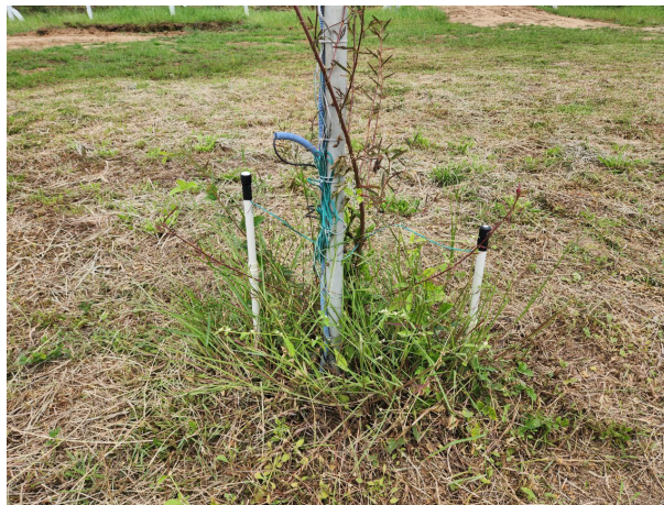
Figure 1: Soil moisture sensors at a single location at two different depths (15cm and 30cm).
