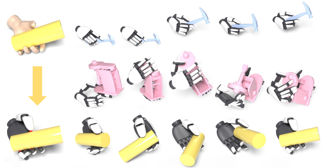
Figure 1. ConTrack tracks long-horizon, contact-rich dexterous hand motion across tool use, articulated object interaction, and in-hand rotation. Adaptive task-style control balances object tracking, hand motion, and contact fidelity.
