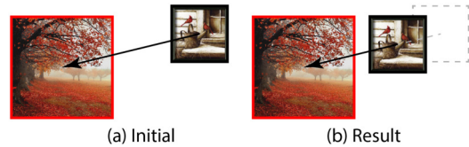
Figure 13: Snapping example. (a) The user drags an art item, which is (b) snapped toward the center of its neighbor item until a minimum spacing between the two is reached.
