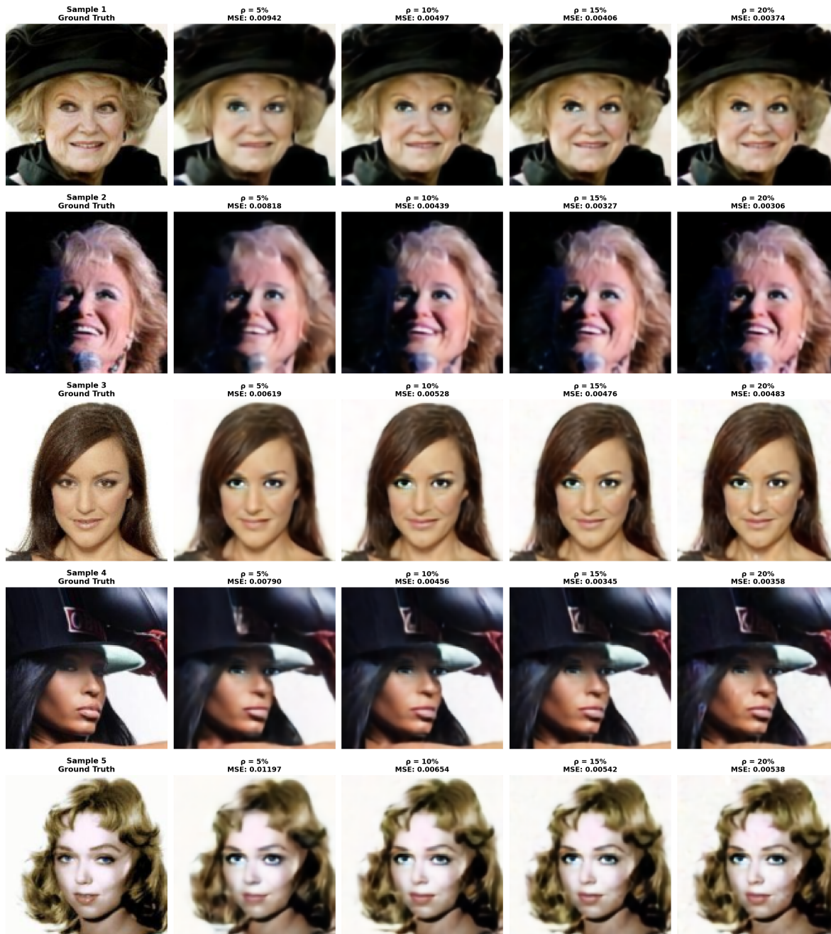
Figure 4: Sparse face reconstructions under increasing observation rates \rho (5% – 20%), showing consistent visual improvement, and decreasing MSE.
